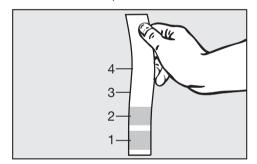
Place the test strip under your kitchen tap for a second and shake off any remaining water. The result is visible in about 1 minute. The appliance can be set to one of 4 hardness levels:
